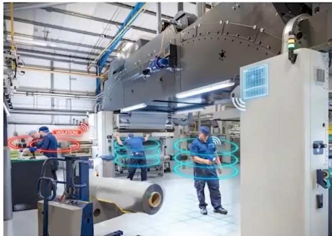
RTLS – Real-Time Locating System
